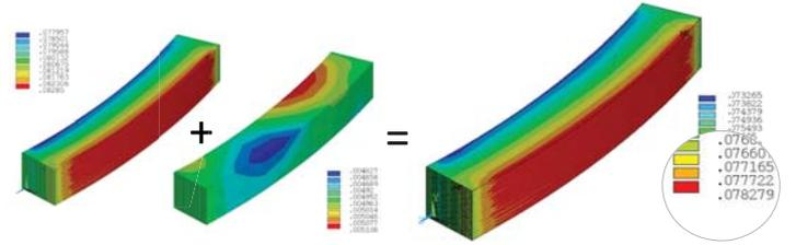
Cool Down (compression) + Lorentz Forces (traction) = Total max Displacement 7,8 cm
