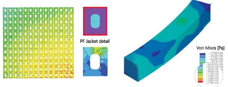
(LHS): full detailed cross section PFC analysis – (RHS): 20 degree 3D sector PF#4 model
