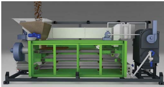
The convective sludge dryer: hopper, multilayer conveyor belt, air diffuser, and burner.
