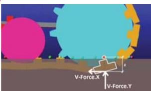
The track-terrain interaction is considered implementing a moving ground model within the MTB environment. It consists of a contact model which follows each rigid link applying a force depending on the terrain characteristics and local link sinkage.
